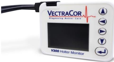
The device has a simple human interface consisting of an LCD and a keypad containing ▲<up>, ▼<down>, ◀<left>, ▶<right> and ↵ <enter> keys. There is also an <EVENT> button for the patient to note significant times during the monitoring period as instructed.
