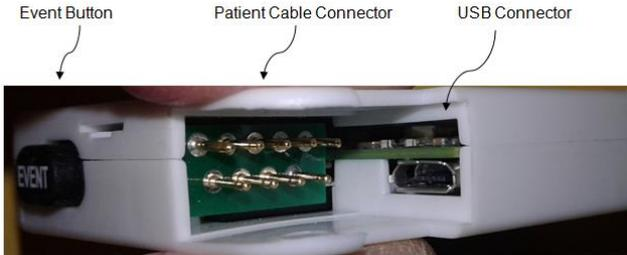
The USB cable is 'polarized' meaning that it can only be inserted one way – Do Not force the cable in, you may need to flip the connector over to insert it. The display on the monitor will change once inserted, and you may hear Windows beep indicating that it 'found' the holter monitor. Once inserted, you can turn your attention to the Trillium Holter Analysis software to complete the transfer.
